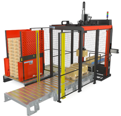
Robot palletiser with pallet magazine adjustable for different pallet widths, front feeding of empty pallets, and automatic pallet exchange
