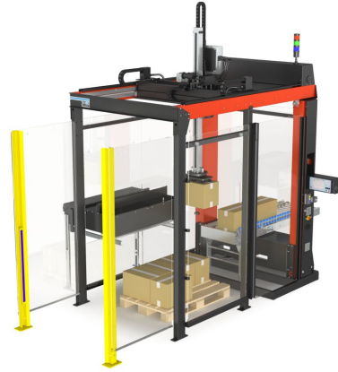
Robot palletiser, pallet on the floor, safety light barrier and with layer pad magazine (1)
